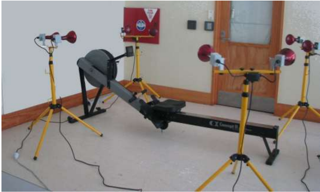
Figure 6.2 Physical representation of the experimental environment. Lighting rig in position fitted with warming bulbs set at a neutral height and direction (additional recording equipment is not pictured).
