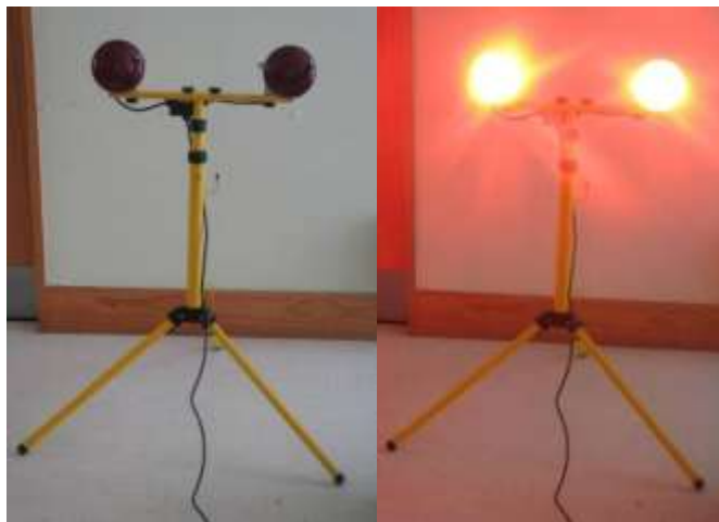
Figure 6.3 Physical representation of the experimental environment. Lamps fitted with warming bulbs set at a neutral height and direction.
