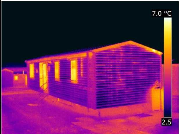
C10 Heated, following pressurisation test, with heat flux sensor placements
