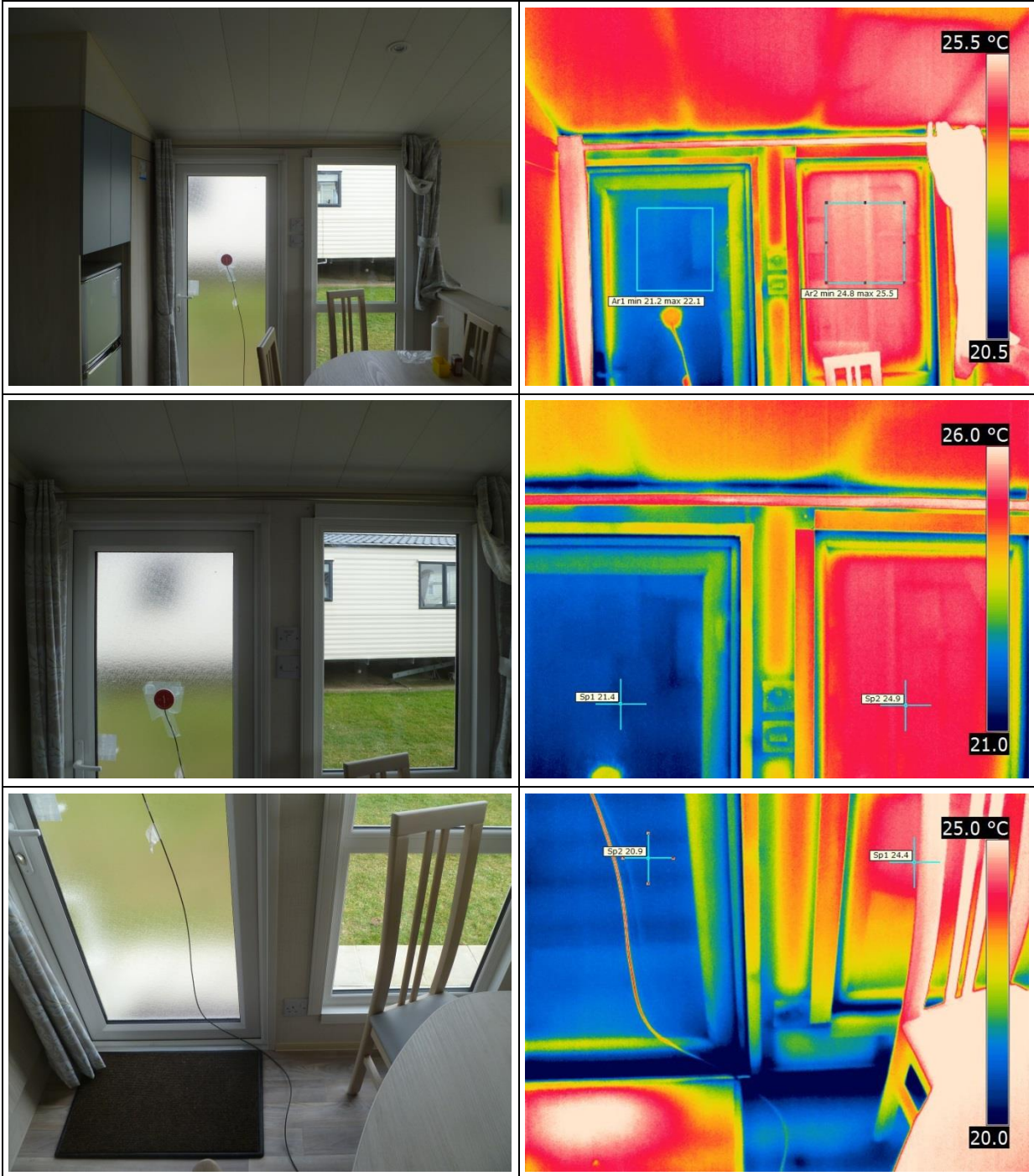
Direct comparison of the original door and a replacement window in C05:
