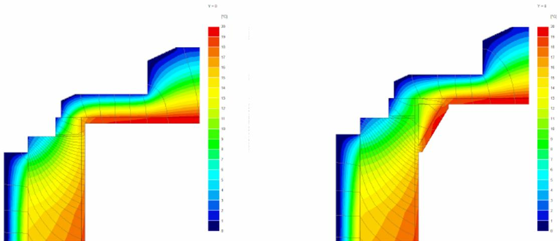
*Figure 7 EWI with and without insulated coving (profile 6)*
