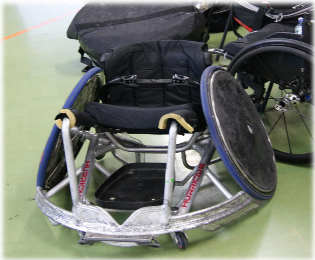
Figure 3: Offensive wheelchair with rounded front for manoeuvrability
