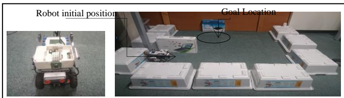
Fig. 2. Left: A snapshot of the built robot with its sensors, actuators, and camera module. Right: The training environment.
