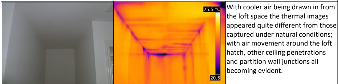
Plot 9 Landing – Under depressurisation
