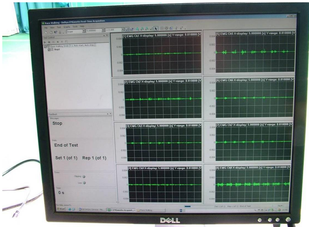
Figure 3.12. EMG data were collected using the acquisition software via telemetry.
