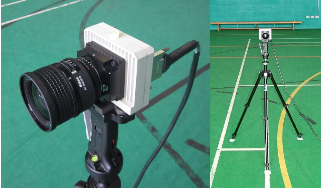
Figure 3.9. The high-speed camera set-up for 2D recording.
