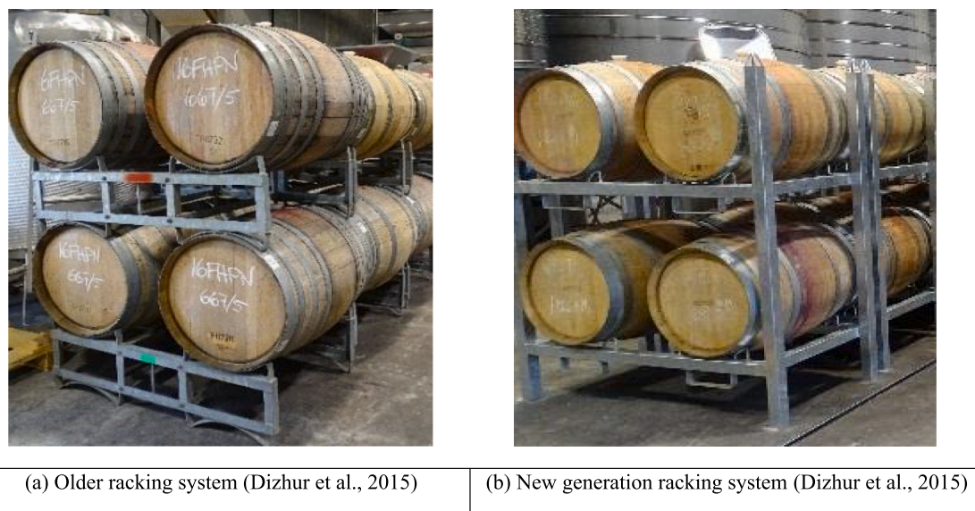
Fig. 3. Two generation of racking system.
