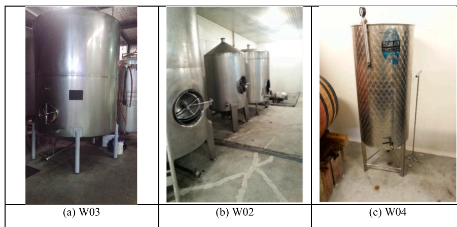
Fig. 5. Slender and small legged tanks used in wineries (W).
