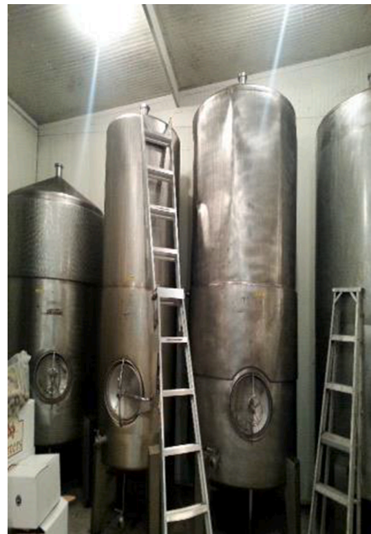
Fig. 15. Ladders used to access top of storage tanks.
