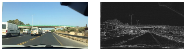
Figure 23: Application of Laplacian filter to a driving image in this research.
