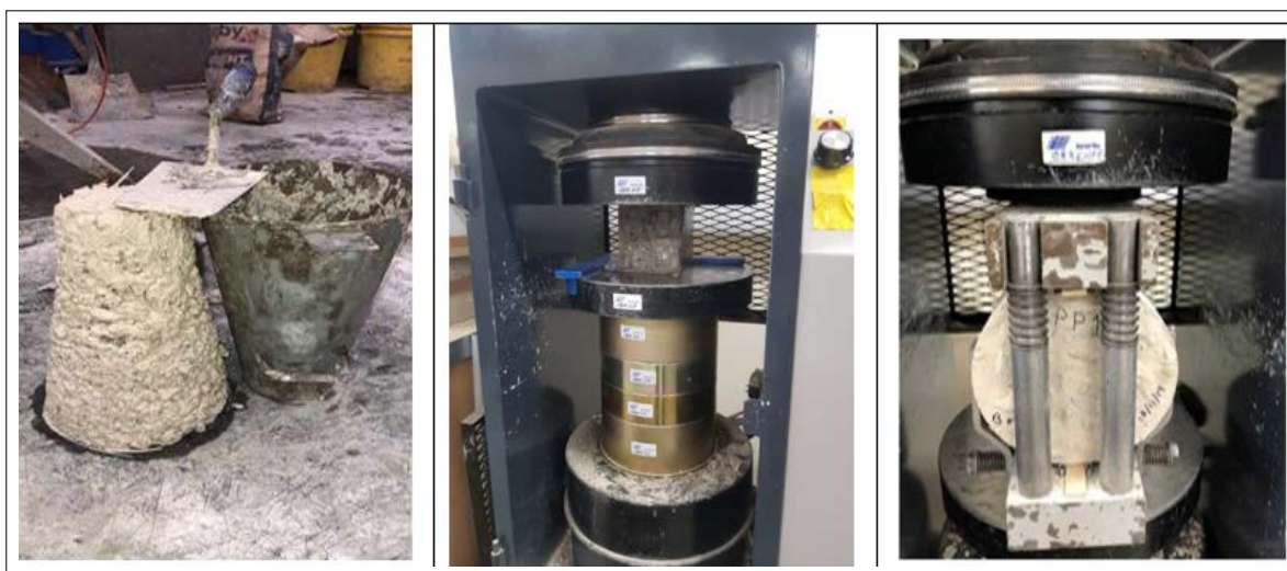
Figure 4a: Slump Testing [48].
