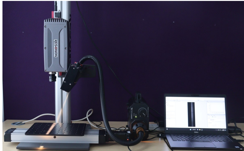
Figure 2. Hyperspectral image data acquisition setup.
