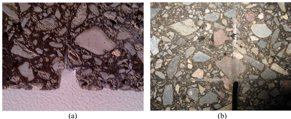
Fig. 2. Notch patterns for specimens: a) with limestone aggregate b) siliceous aggregate.
