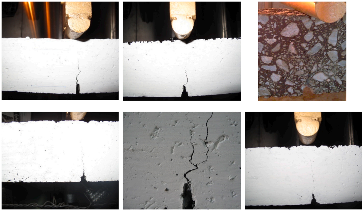
Fig. 5. Samples used for cracked beam annotations.
