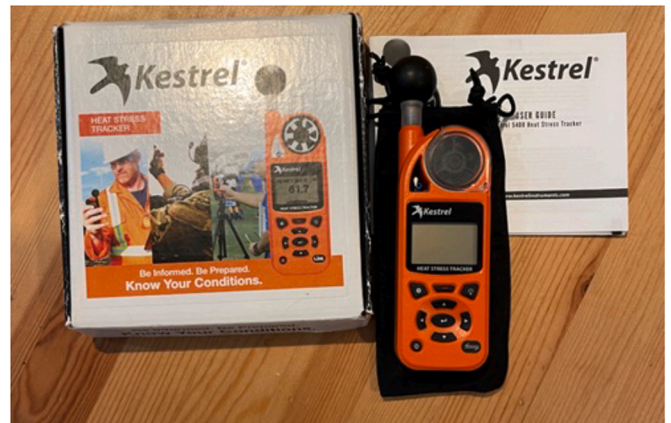
Fig. 3. Kestrel 5400 Heat Stress Tracker used for air temperature measurements.
