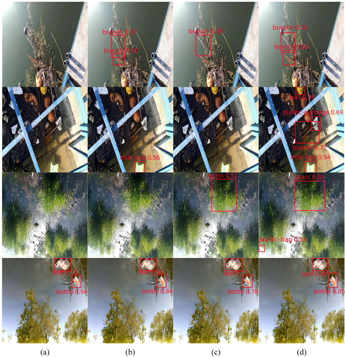
Fig. 6. Detection results for the dataset are presented as follows: (a) for YOLOv3, (b) for YOLOv5, (c) for YOLOX, and (d) for EC-YOLOX.
