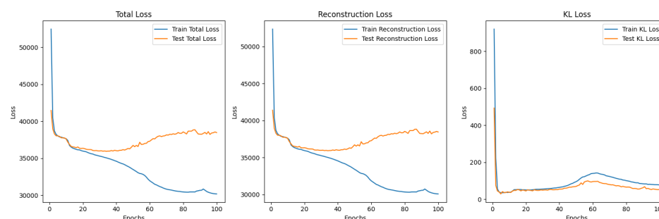
Figure 21. Loss functions for the dataset of band 151 images using \beta = 0.1 to \beta = 1 for 100 epochs. The training loss for the Total Loss and Reconstruction Loss continue to decrease while the test loss for both increases after approximately 25 epochs. This indicates that the model is overfitting. The KL Divergence for both the training and test dataset appears to be slowly increasing, then at approximately 60 epochs, they begin decreasing. The Total and Reconstruction Loss curves appear similar to one another but the KL Divergence loss curves do not.
