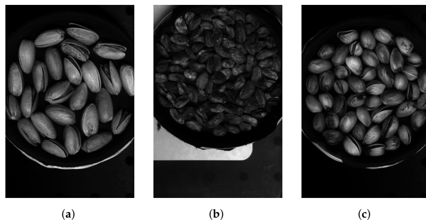
Figure 5. Representation of the 453.8 nm wavelength at the 3 different aflatoxin levels: (a) Less Than 8 \mu\text{g}/\text{kg} , (b) Greater Than 160 \mu\text{g}/\text{kg} , and (c) Greater Than 300 \mu\text{g}/\text{kg} .
