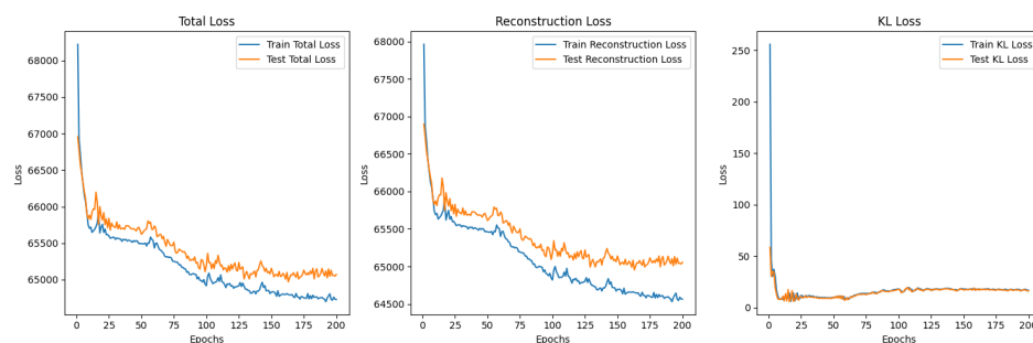
Figure 28. Loss functions for the dataset of band 361 images using \beta = 1 to \beta = 10 for 200 epochs with batch size 100. The training and test loss for the Total Loss and Reconstruction Loss decrease. The KL Divergence for both the training and test dataset appear to be increasing at a decreasing rate, indicating that they may begin the decrease and converge to a loss of 0.
