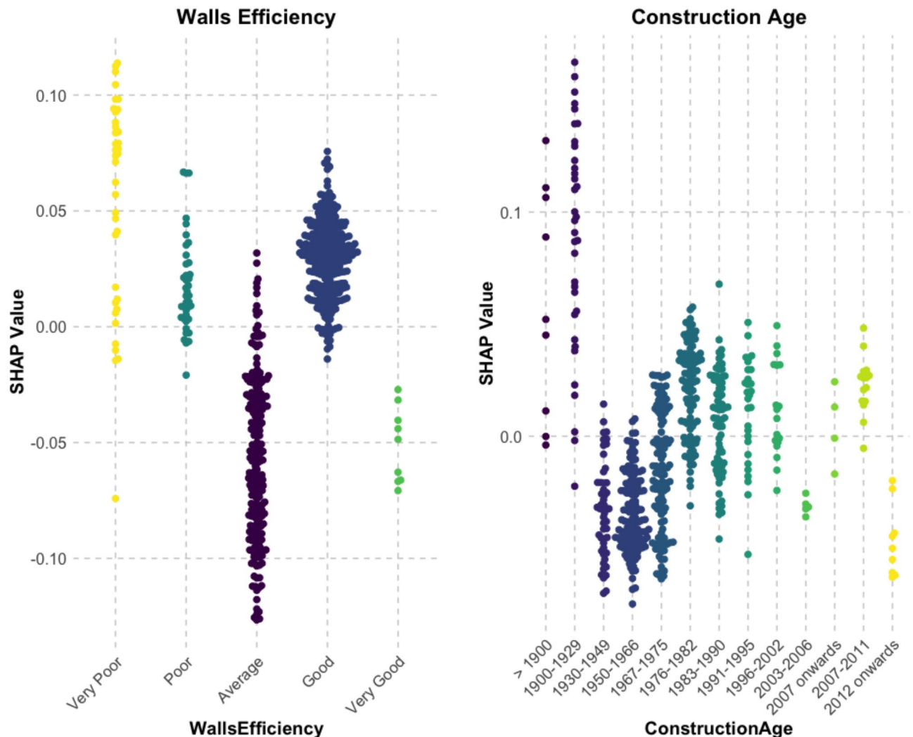
Fig. 4. SHAP Value Distributions for Wall Efficiency and Construction Age: Positive values indicate higher damp risk, negative values indicate lower risk, and larger magnitudes reflect stronger predictive influence.
