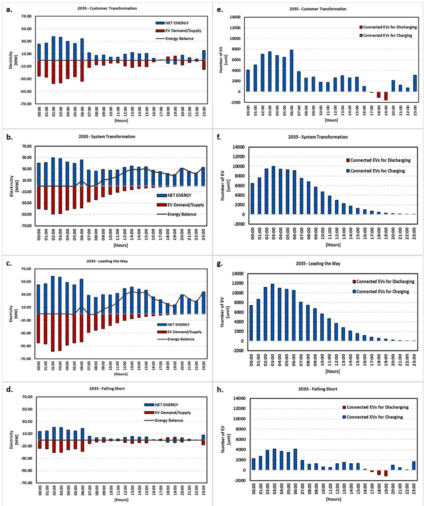
Fig. 9. Energy and EV connection profiles for the selected day in 2035: Panels (a-d) comparative analysis of net energy, EV demand/supply, and energy balance across scenarios; Panels (e-h) the temporal distribution of EVs connections for charging and discharging operations.
