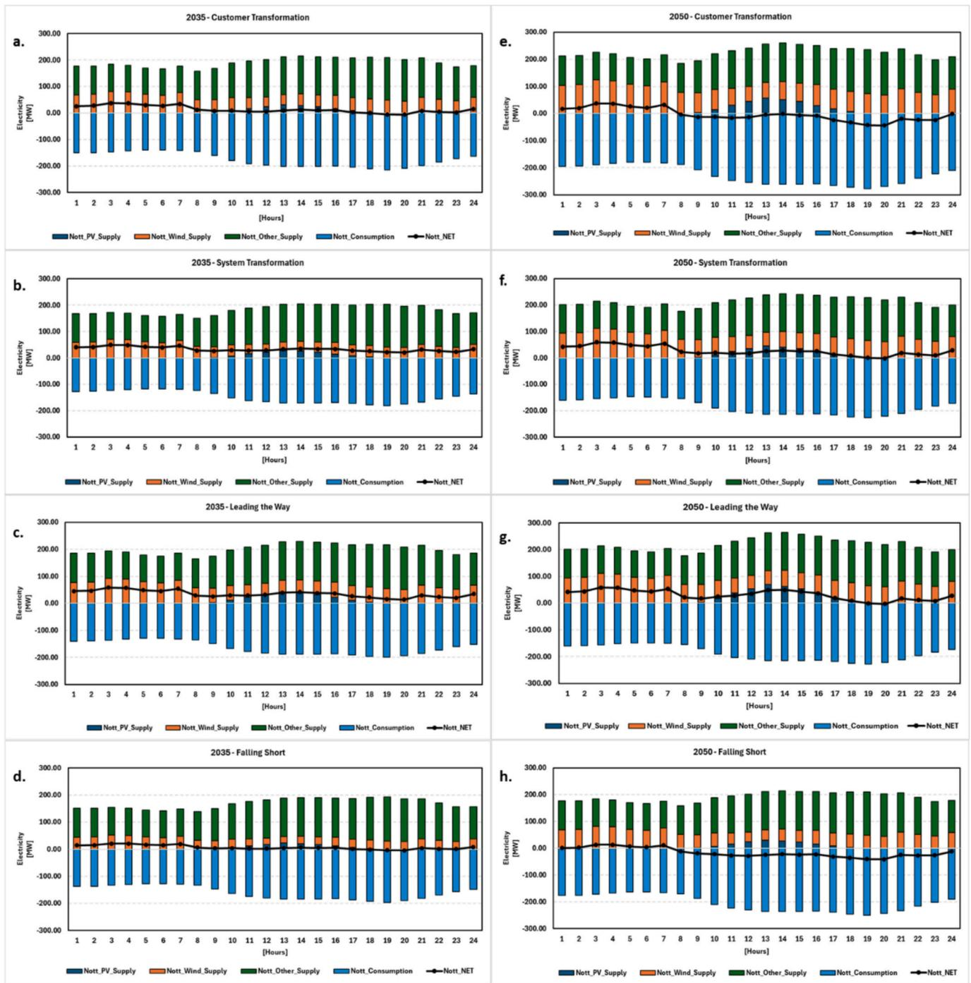
Fig. 8. Hourly net energy profiles for the selected day under different scenarios in 2035 and 2050: a-d) 2035 (Customer Transformation, System Transformation, Leading the Way, Falling Short), e-h) 2050 (Customer Transformation, System Transformation, Leading the Way, Falling Short).
