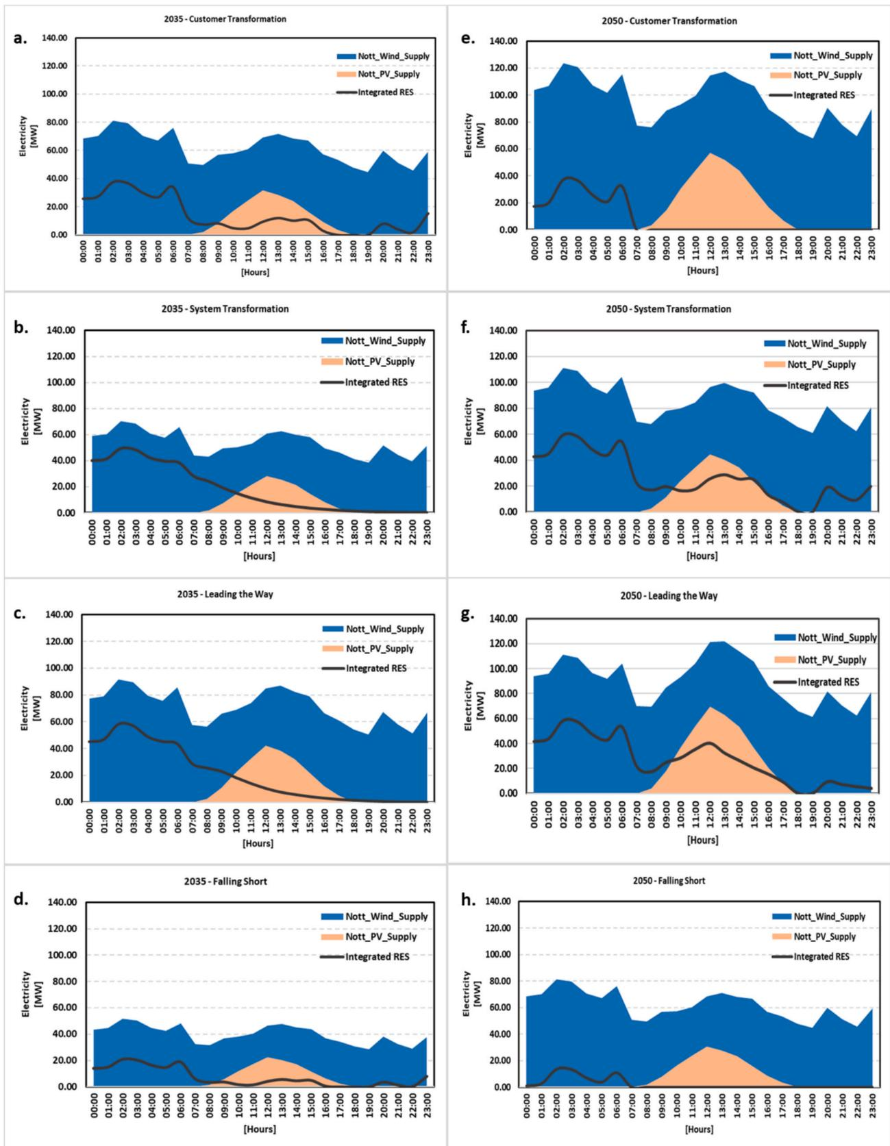
Fig. 11. Hourly profiles of wind and PV energy vs integrated RESs through EV charging operations on a representative day: Panels (a-d) for 2035; Panels (e-h) for 2050.
