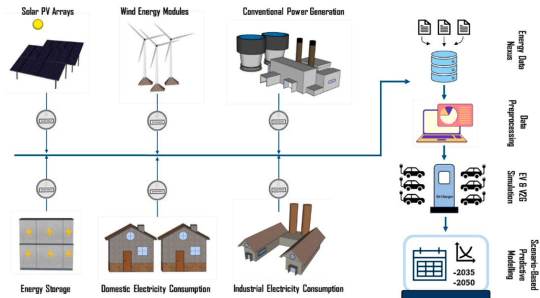
Fig. 1. A systematic overview of the methodological framework with RESs, EVs and grid dynamics.
