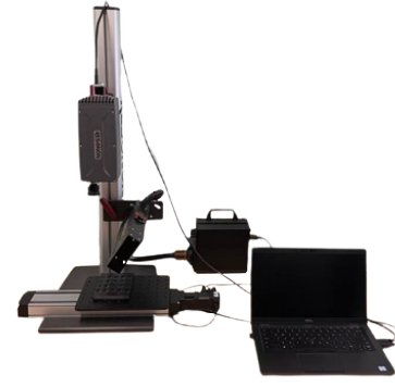
Fig. 1. Resonon Benchtop hyperspectral camera setup for lab analysis, featuring a camera, adjustable stand, light source, and computer for data acquisition [22].
