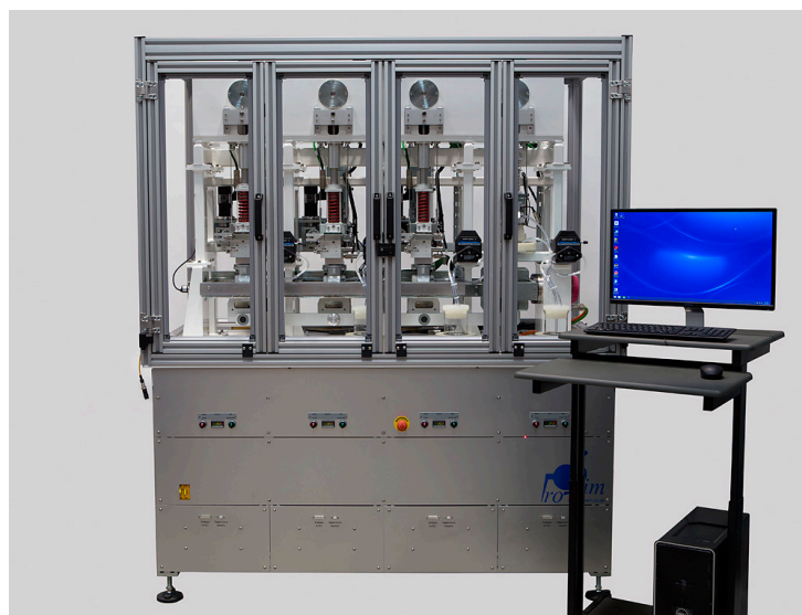
Figure 1. A three-station Prosim Hip wear simulator (Simulation Solutions, UK) combined with a load soak.
