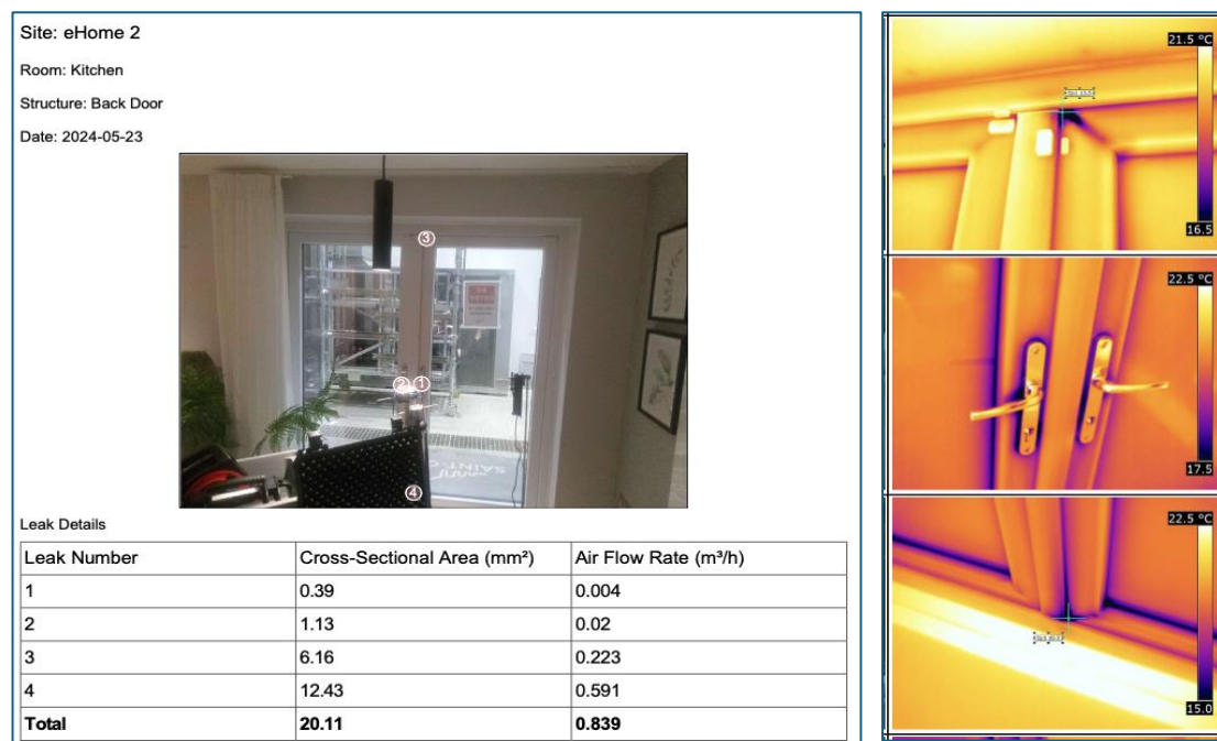
Figure 6: Excerpt from the Portascanner® AIRTIGHT 2.0 automated report at Salford Energy House 2.0, alongside the corresponding thermographic results.
