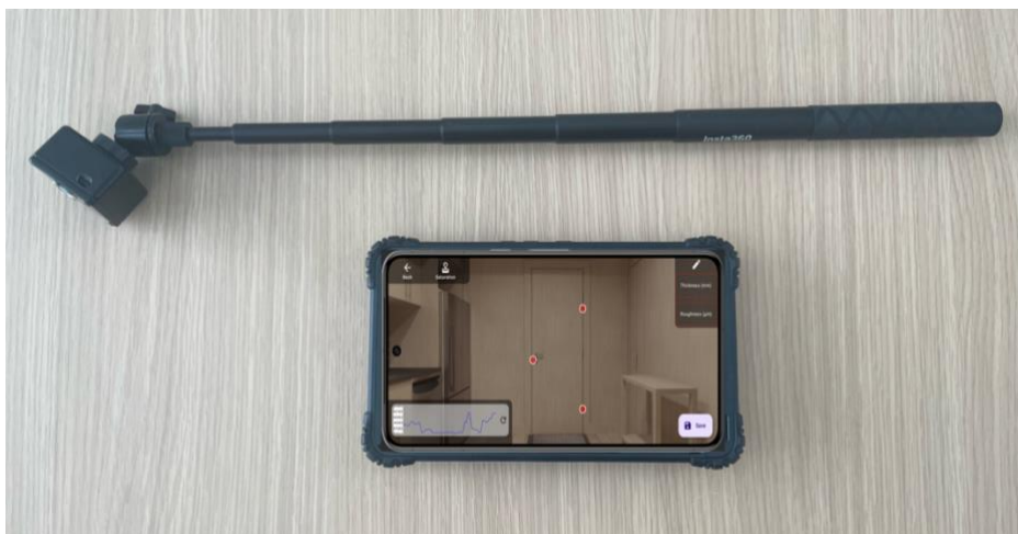
Figure 1: The Portascanner® AIRTIGHT 2.0, ultrasonic sensor and tablet
