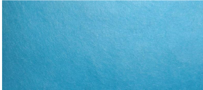
Figure 2.2 Blended sample number 2.23 with a mean colour difference of 15 CIELAB \Delta E (1:1 scale)
