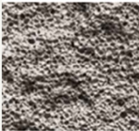
Figure 1: Cellular structure of Aircrete with levels of porosity up to 85%.
