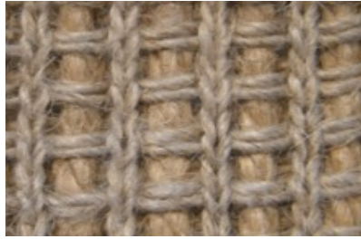
Figure 5: Sisal inlay/knitted flax 1x1 rib base structure
