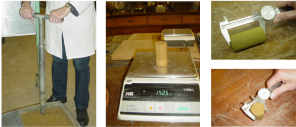
Figure 17.11: Linear density method
