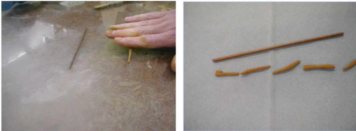
Figure 17.8: Plastic limit test
