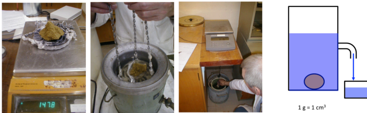
Figure 17.12 Immersion/Displacement in water – density methods
