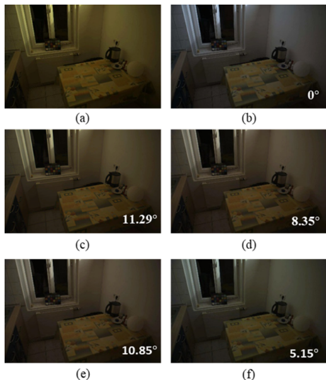
FIGURE 5. A sample image from Gehler and Shi dataset [48]: (a) original image, (b) ground truth, (c) Gray Edge-1 [11], (d) Weighted Gray Edge [12], (e) CNN [28] and (f) proposed method.
