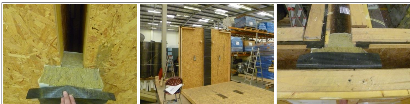
Figure 64 Test 4.19, ARC T-Barrier, 100 mm party wall, 100 mm external wall
