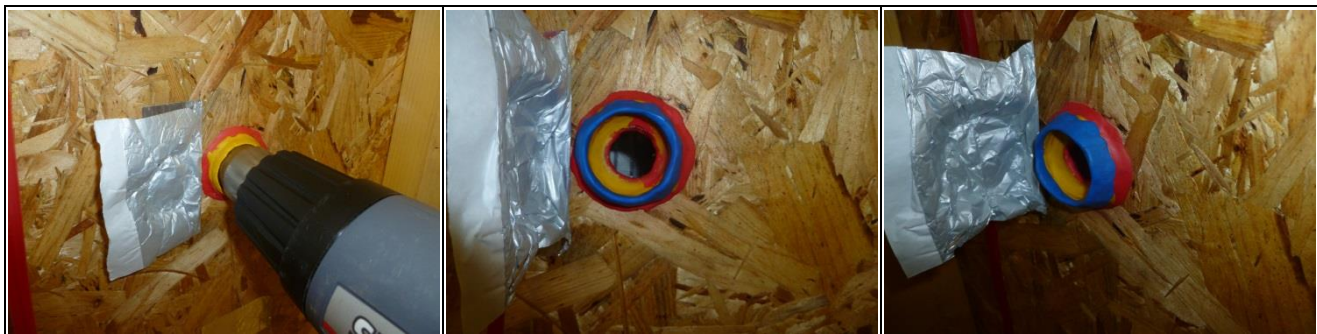
Figure 29 Original seal at the injection point and following the application of additional Sugru™ following test 3.7
