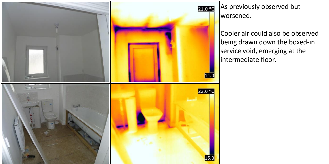
Bathroom – Under depressurisation
