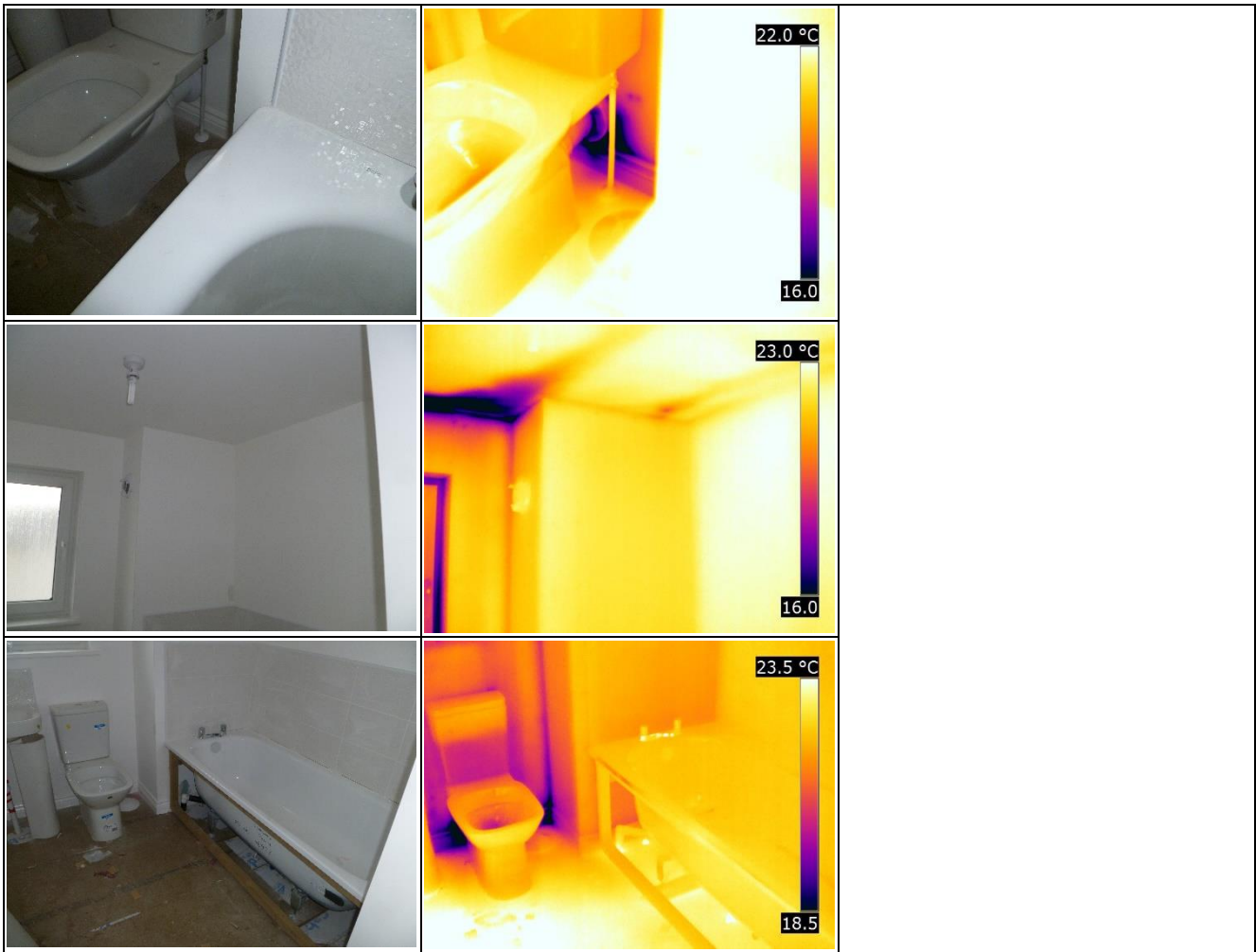
Bathroom – Under depressurisation
