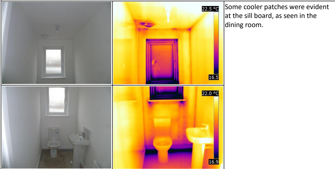
Ground Floor WC – Under depressurisation
