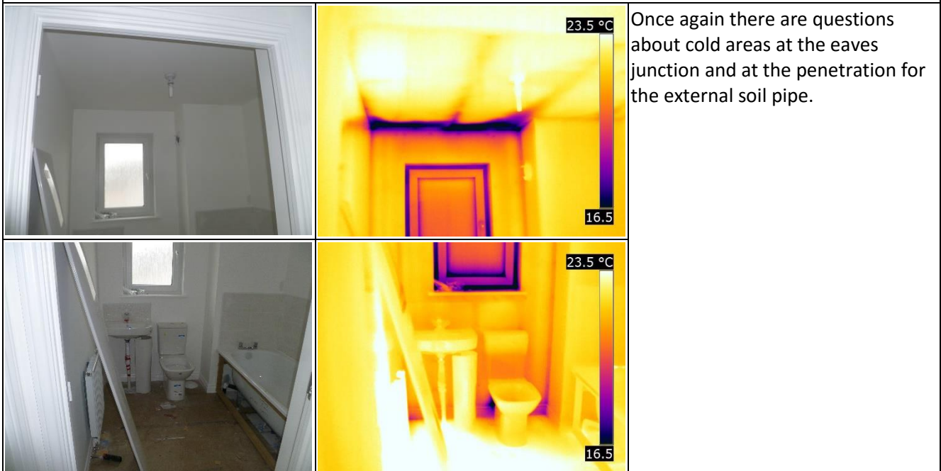
Bathroom – Under natural conditions
