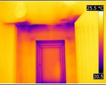
As seen previously there are colder patches at the eaves junction; these appear cooler than the window frame, and if condensation forms in the bathroom it will form on the coldest surfaces first, so may cause future issues.
