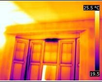
Again, the external wall appeared marginally cooler at the bottom than was expected from just the natural temperature stratification in the room and the fact that the top part of the wall reflected the warm ceiling and the bottom part reflected the colder floor. The bay roof again showed minor cooler spots along the lines of the external wall above. There was also some noticeable cold air infiltration at the bay window without any
