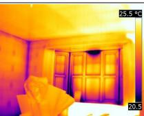
The bay ceiling appeared to show a colder section, but this was difficult to see due to the trickle vent being open beforehand and the reflection of the glazing.
