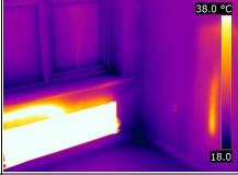
Again, the external corner where the gas meter box was positioned was noticeably cooler than the surrounding areas, even considering corner effects of the thermal imaging (where colder surfaces are reflecting each other making the internal corners appear cooler than they actually are).
