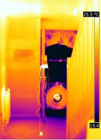
Under depressurisation it appears that colder air is being drawn into the boxed-in service void, as differing wall temperatures can be seen below the consumer unit.
