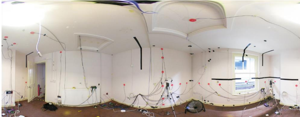
Figure 2. Typical experimental set up in the test house (red disks show in situ U-value measurement locations)
