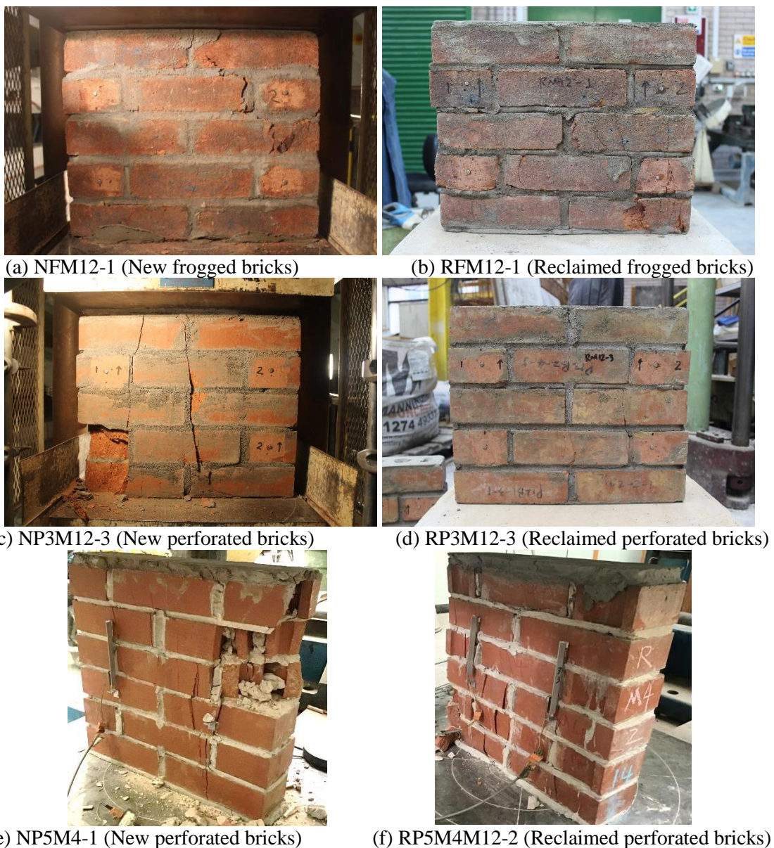
Figure 8 Failure modes of wallettes
