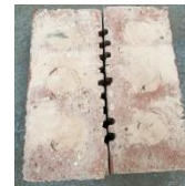
(c) Reclaimed bricks by punching with mortar infilled
