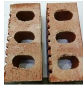
(b) Reclaimed bricks by punching without mortar infilled
