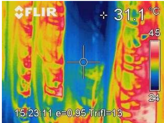
Figure 7: Hotspots (red) and loss of cold air (blue) in the central area.
