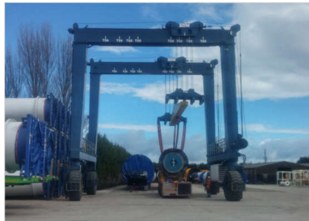
Figure 7. Configuration of the experiments to validate the proposed regression model: Crane, trailer and load.
