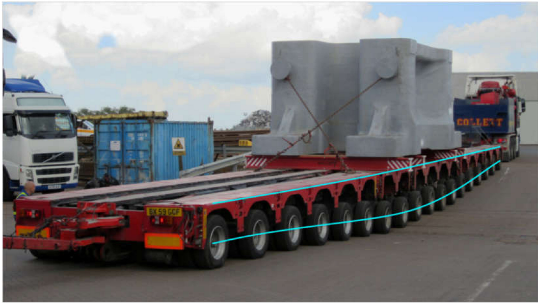
Figure 1. Modular trailer axle compensation [28].
