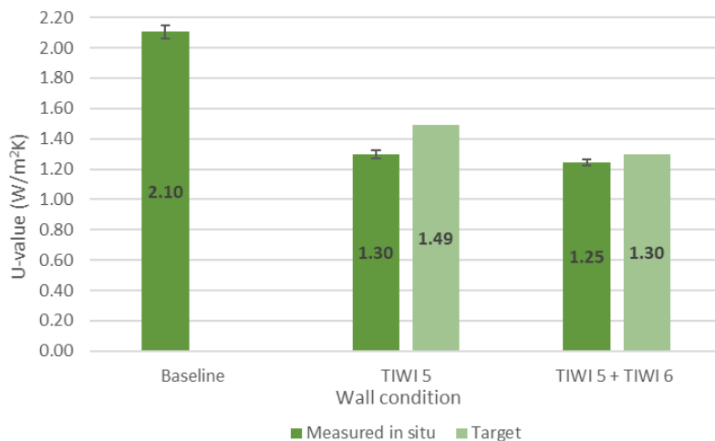
Figure 3-7 Mean in situ U-value and retrofit target U-values for the test wall of House C in each condition
