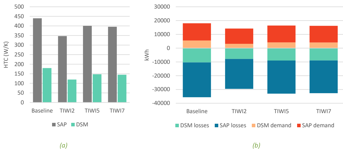
Figure 4-16 House C: comparison between HTC (a), and heat losses and heat demand (b) in the RdSAP and DSM calculations
