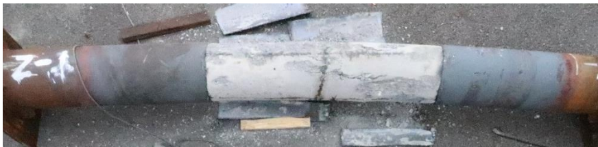
(a) Circular steel tube after being cut open
