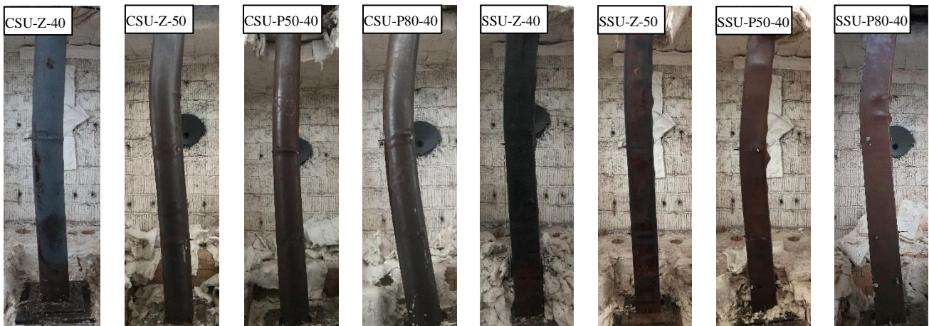
Fig.6. Failure modes of the specimens
