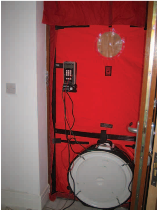
Pressurisation equipment fitted in the front door opening – internal view showing fan and controller
