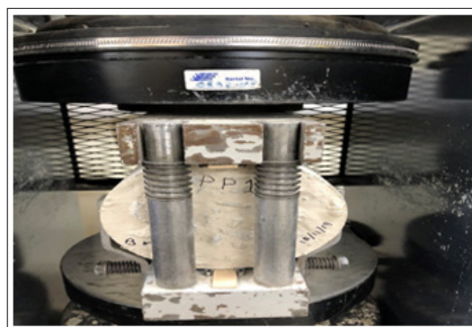
Figure 2: Cylinder Testing for Tensile Strength
