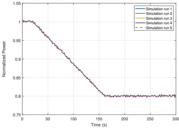
FIGURE 3. Reactor power in the presence of bias-type faults in the power sensor.
