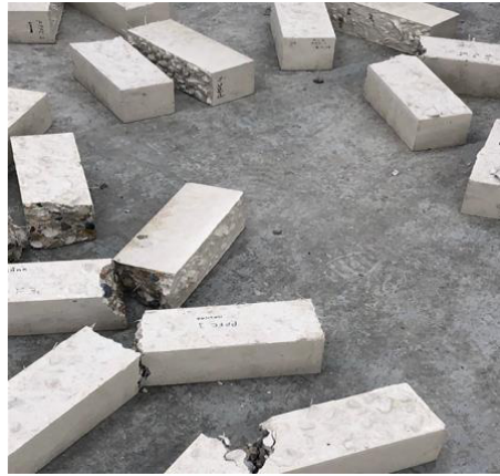
Figure 8: Ruptured prisms after 3-point loading.
