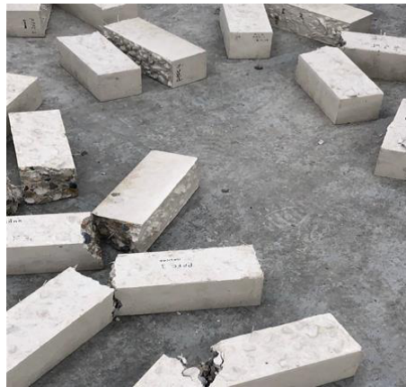
Figure 8: Ruptured prisms after 3-point loading.
