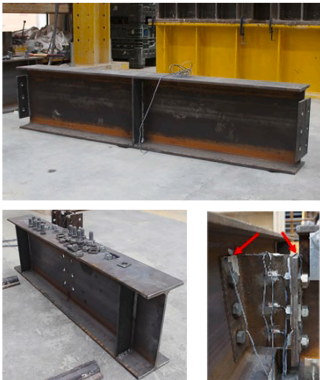
Fig. 9. Dis-assembled steel components after tests and observed bolt slip during the first test.
