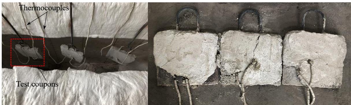
(a) Before fire test
