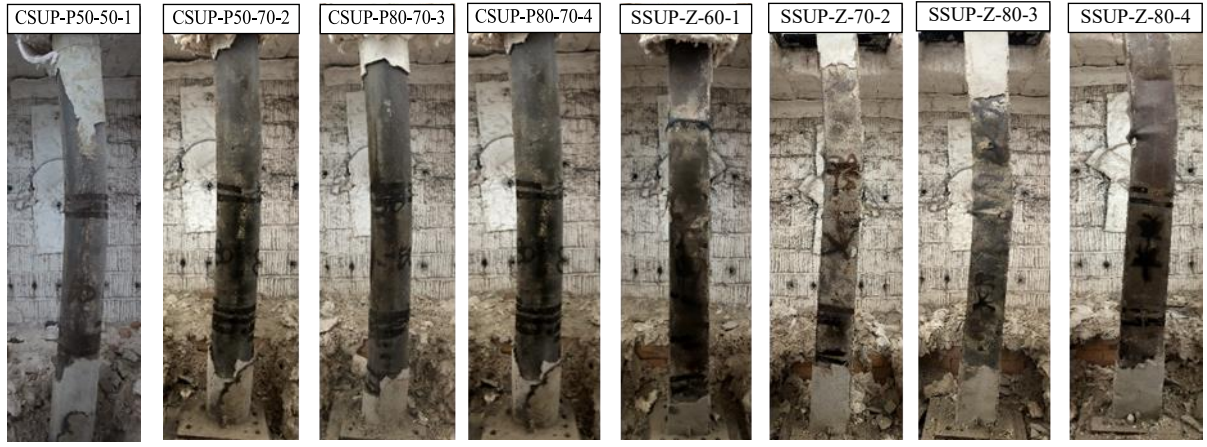
Fig.10 Comparison of failure modes for SRCST column specimens after removing the fire resistive coating (West)
