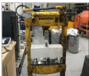
Figure 2: 3-point loading flexural testing machine for 500x100x100 mm prisms/ beams [44]
