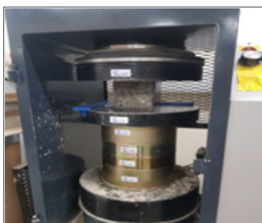
Figure 1: Compressive testing machine for testing of 100 mm cubes (BSI - BS EN 12390-2, 2000)
