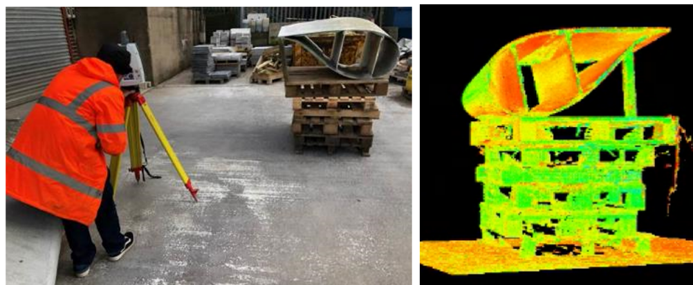
Figure 2. LiDAR scanning of one meter long segments.
