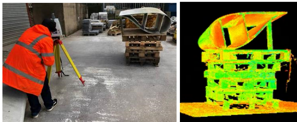
Figure 2. LiDAR scanning of one meter long segments.
